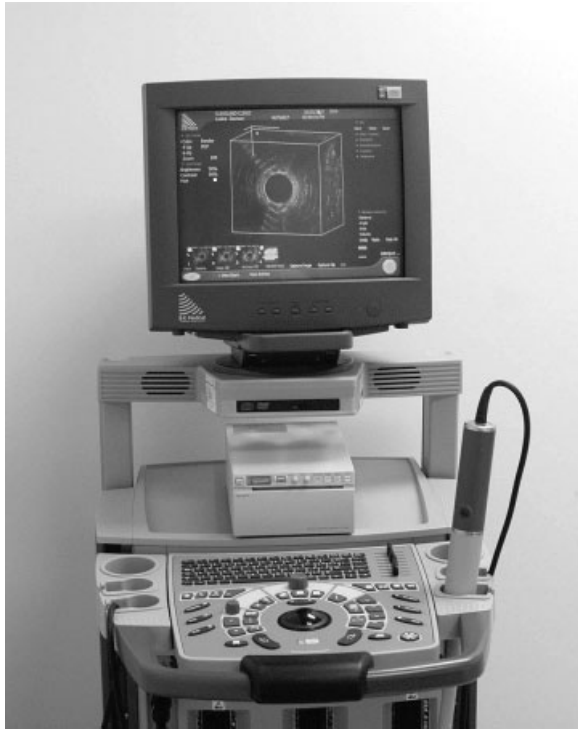
Figure 7 B-K Medical (Herlev, Denmark) three-dimensional (3D) anorectal ultrasound equipment. The data from a series of closely spaced two dimensional images is combined to create a 3D image that can be freely rotated and sliced. The data stored in a file originating from one acquisition can be reviewed many times. Reproduced with permission from the Cleveland Clinic Foundation, Cleveland, Ohio.
